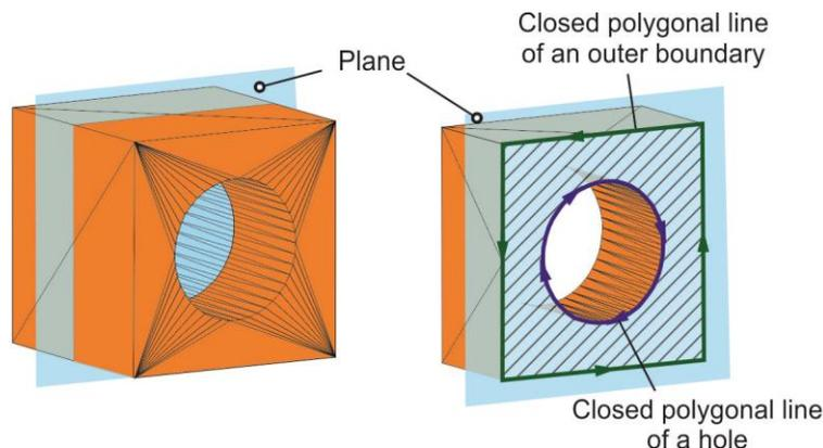
**Figure 7:** Polygons formed by the Polygon Construction algorithm. The hatched area has to be capped.
