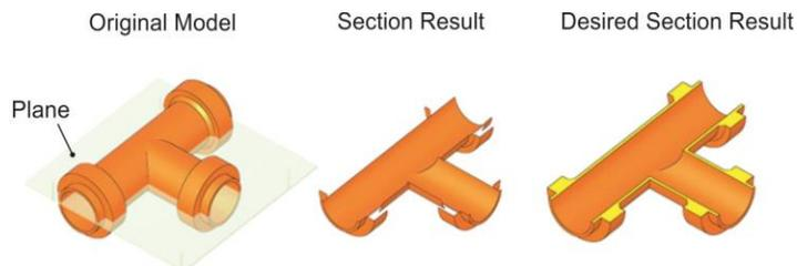
**Figure 5:** (a) Original model, (b) Section result without capping open areas, (c) Desired section result.
