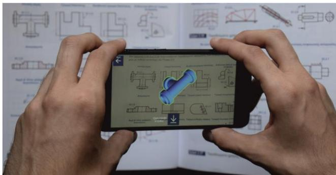
**Figure 1:** Selection of a 3D model through Augmented Reality based on textbook marker.
