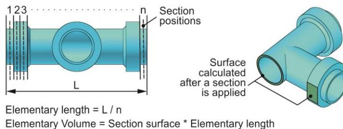
**Figure 3:** Calculation of Model's Volume.
