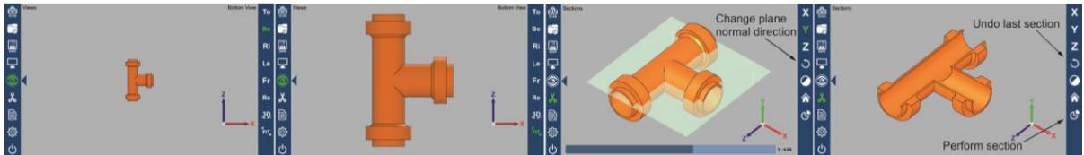
**Figure 2:** (a) Bottom View, (b) Fit Function, (c) Section in Y axis, (d) Section Result.
