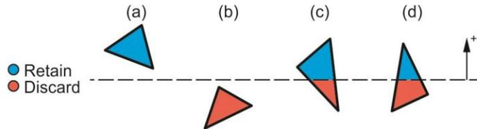
**Figure 6:** Main cases a triangle may be located in respect to the section plane.
