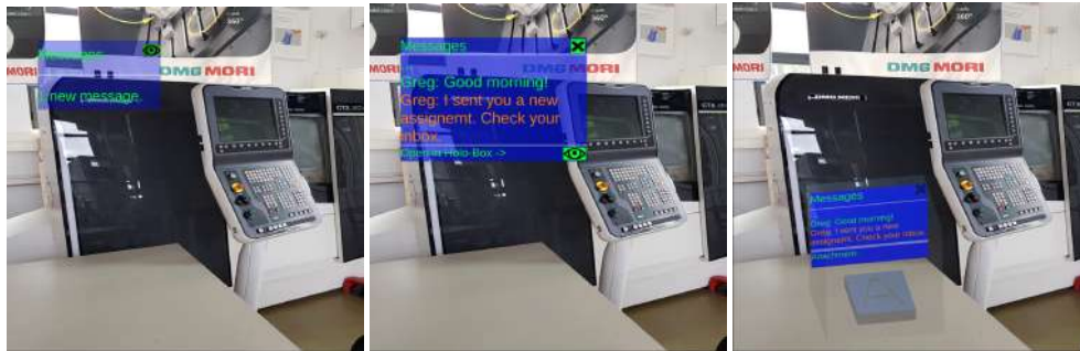
Figure 1: From left to right: The Holo-Box interface's three Levels of Detail, shown in the context of a machine shop. Simple Glanceable (SG-level 1), Detailed Glanceable (DG-level 2) and the Interactive Holo-box (HB-level 3).
