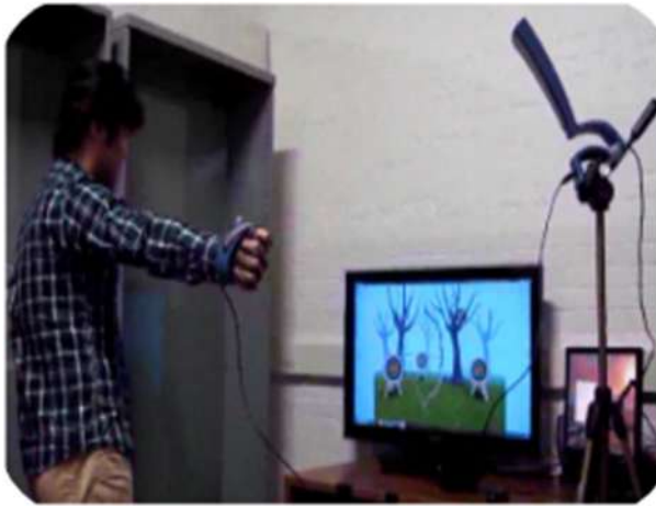
Fig. 5 Use of Kinect in conjunction with p5 glove [8]
