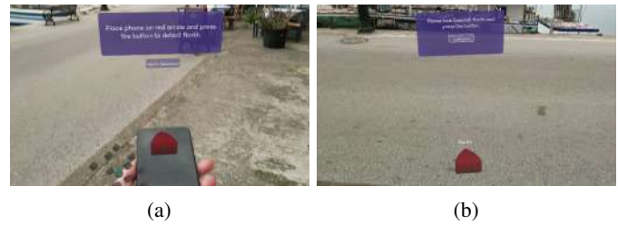
Fig. 2: Calibration process: (a) Phone placed on the pointer object to record its heading direction. (b) The pointer object is rotated accordingly facing the north direction.
