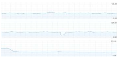
Fig. 13: (Up) Frame rate while the navigation feature with the 3D map is enabled (38-45 fps). (Middle) Quick frame rate drop when the user presses a map pin (18-20 fps). (Down) Frame rate when water is rendered ( \sim 30 fps).
